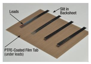
Protection of the backsheet from impression from leads during lamination. A small tab of a release material is placed under the leads prior to lamination.
