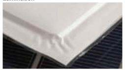
More conformable backsheet allows for a good seal, faster air bleed cycle and reduced EVA contamination.
